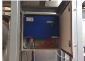
SOFO Fiber Optic Sensor Datalogger
