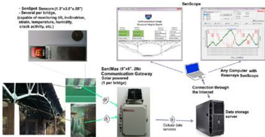
Illustration of a complete bridge health monitoring system based on SenSpot sensors
